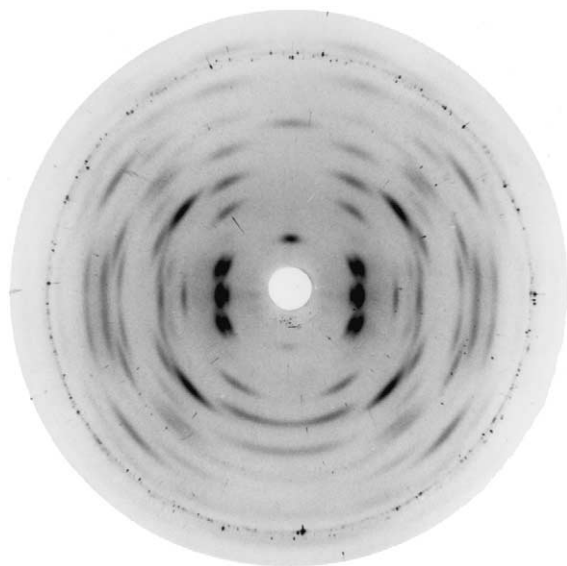
Fig. 1. X-ray diffraction pattern from a polycrystalline and oriented specimen of the sodium salt of beijeran using Cu K \alpha radiation of wavelength 1.5418 Å. The fiber is tilted from the vertical direction by 14°. The ring corresponds to 3.035 Å spacing characteristic of calcite.
